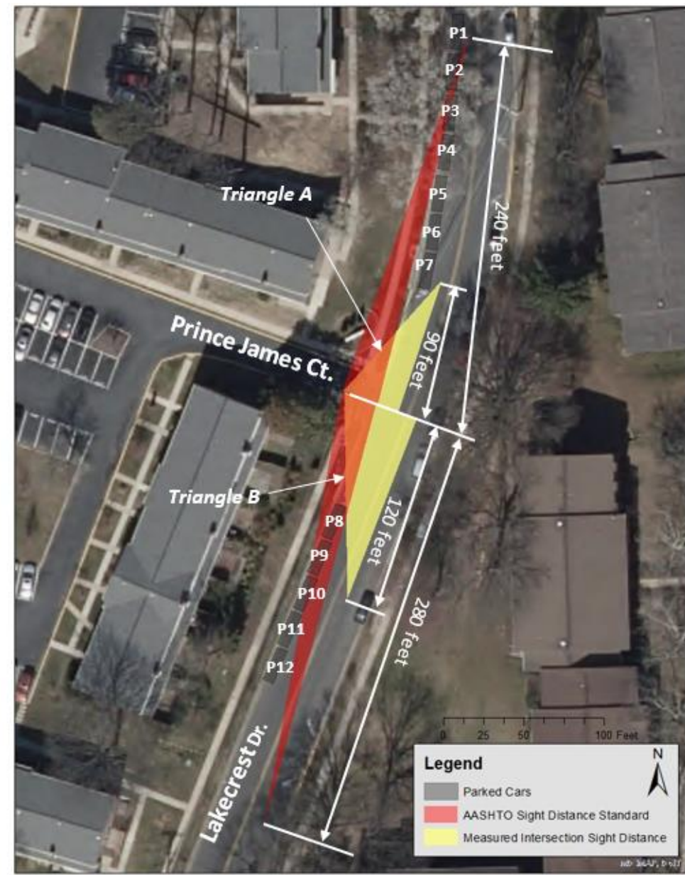
Figure 4 – AASHTO Intersection Sight Distance vs Measured Intersection Sight Distance
