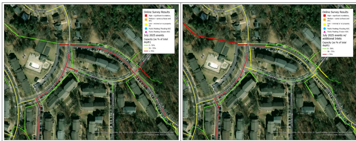
Figure 14. Road Flooding (shown in red in left panel) Due to Inadequate Storm Drain Inlet Capacity at Lakeside & Westway.
